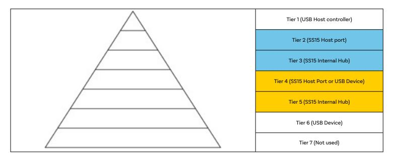
From this you can see we can connect 2 hubs in a daisy chain fashion and still connect USB devices to both hubs, if we were to connect a 3rd hub the hub would connect but you wouldn't be able to connect any USB devices as you will have run out of tiers.
