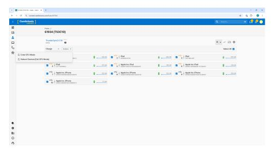
Simply select Enter DFU Mode and then type in the confirmation phrase, and the command will be sent to all connected devices, enabling DFU mode with ease and efficiency. The name of the devices will change to show that they are now in DFU Mode. This streamlined method ensures a smooth experience for managing multiple devices
